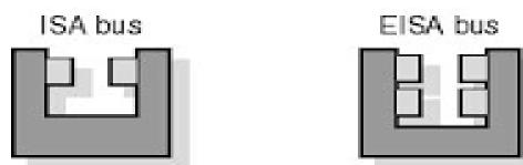
➢EISA is completely compatible with ISA cards since the EISA connectors were deeper and the additional contact rows were placed below the ISA contact rows.
