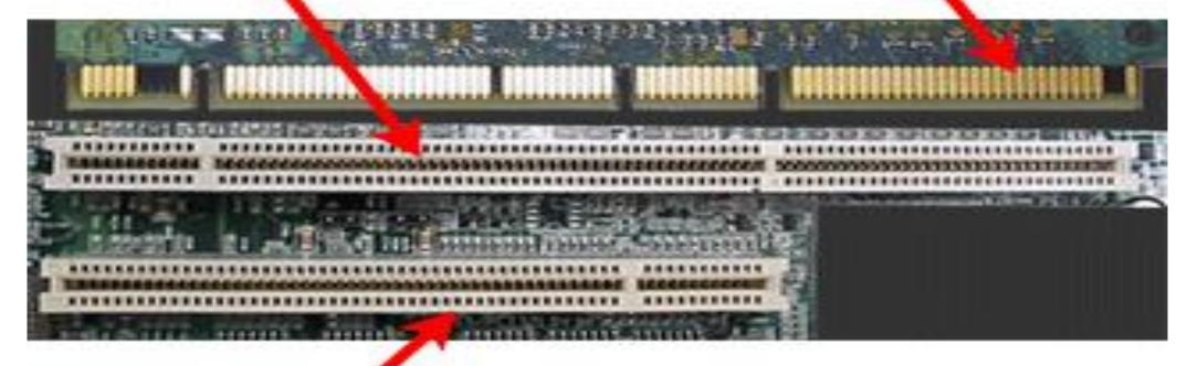
PCI Slot (32-bit/33MHz)
